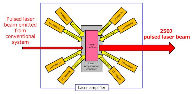
%The laser medium is pumped by LD modules and stores energy. When a pulsed laser beam passes through the laser medium, it receives energy from the laser medium and boosts the output power.
