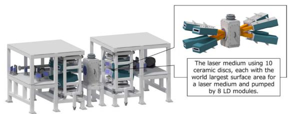
Fig. 2 Structure of newly developed pulsed laser amplifier
