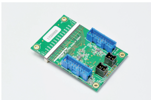
Silicon photodiode module coupled with scintillator used for baggage inspection
