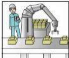
▲ Illustration of application of photo ICs. Photo ICs are used in applications that include controls for robotic arms and detecting passing products.
