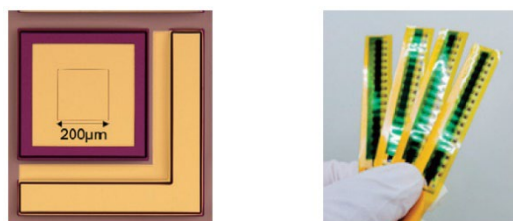
▲Newly developed photonic crystal surface emitting laser (left) and flexible organic optical sensor (right)
