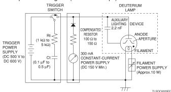
When using the above circuit to operate a deuterium lamp with a 0.5 mm aperture, setting the trigger resistance to 1 k $\Omega$  and the trigger capacitance to 0.5  $\mu$ F as the CR constant is recommended in order to ensure reliable lamp ignition.
