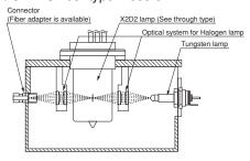
\* Power supply for lamp operation should be prepared
