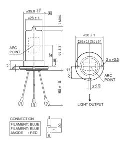
Tolerance of emitting point (center) With respect to axial line A: ±0.1 With respect to plane B: ±0.1
