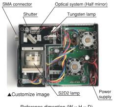
Reference dimention (W  $\times$  H  $\times$  D) : 72 mm × 40 mm × 90 mm
