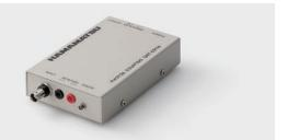
The photon counting unit C9744 converts single photoelectron pulses from a photomultiplier tube into digital signals of logic pulse by use of the built-in amplifier and discriminator circuits.
