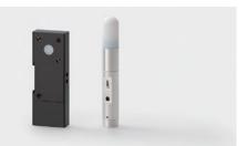
The L11416 and L11494 series are LED light sources mainly designed for adjusting the sensitivity of PMT (photomultiplier tubes) and PMT modules. The L11416 series is a test tube type easily mounted in lab devices such as for blood sampling, while the L11494 series is a plate type designed to be placed on a sample stage.
