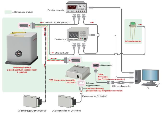
\*1: The name printed on the power cable attached to the product. Refer to "Power connector specifications" on page 4 for the functions. \* The cable connected to the power connector is attached with the product. The cables connected to the DC power supply and the TEC temperature controller have to be manupulated by the user.
