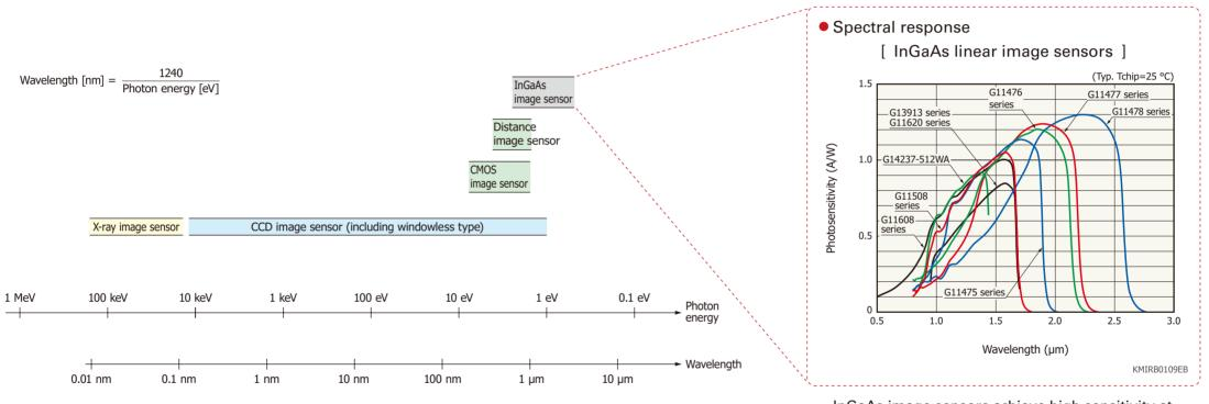
InGaAs image sensors achieve high sensitivity at wavelengths from 0.5 to 2.55  $\mu$ m.
