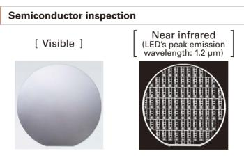
The InGaAs area image sensor is used to detect the patterns of silicon wafers.
