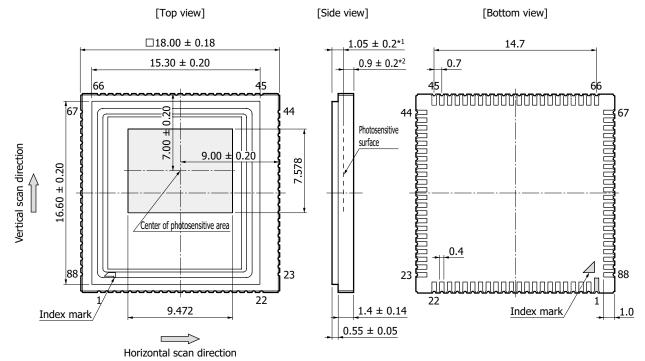
Tolerance unless otherwisenoted:  $\pm 0.2$ Allgle accuracy of effective pixels:  $-2^{\circ} \le \theta \le 2^{\circ}$
