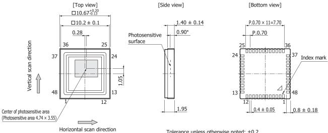
Tolerance unless otherwise noted: ±0.2 Angle accuracy of effective pixels: ±3.15° Weight: 0.5 g
