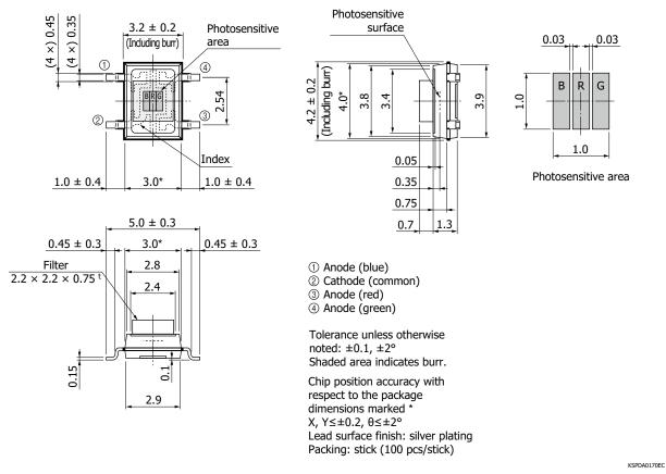
Note: If excessive vibration is continuously applied to the glass filter, there is a risk that the filter may come off, so secure the glass filter with a holder.
