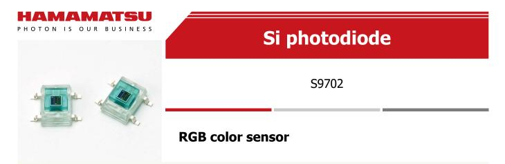
The S9702 is a color sensor molded into a plastic package having a 3-channel (RGB) photodiode sensitive to the blue ( $\lambda p$ =460 nm), green ( $\lambda p$ =540 nm) and red ( $\lambda p$ =620 nm) regions of the spectrum. The S9702 has a 3-segment (RGB) photosensitive area of  $\Box 1$  mm. When compared to the previous model (S9032-02), the S9702 is significantly miniaturized (package size 55% less in cubic volume, PC board mount space 43% less in area).
