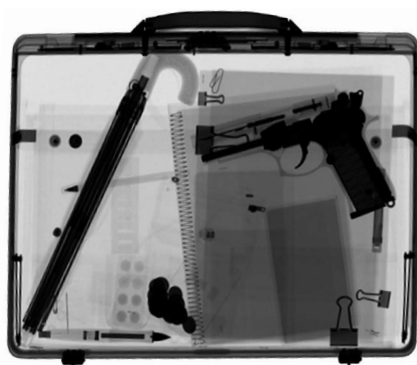
[Figure 2-1] Imaging example of baggage inspection equipment
