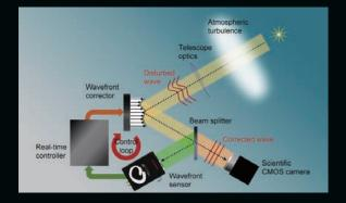
As the phase can be measured directly, errors are less likely to occur. Since adaptive optics for direct imaging of exoplanets requires high-speed and high-precision wavefront control, so does wavefront measurement. Improving the performance of wavefront sensors is essential for the evolution of adaptive optics.
