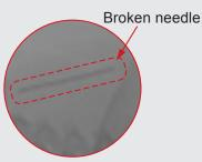
The camera has high detection capability even over a wide inspection field and so can even detect thin foreign matter such as broken injector needles.
