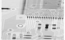
When used along with a microfocus X-ray source, the camera gives sharp images that allow detecting the bonding wire status and solder voids
