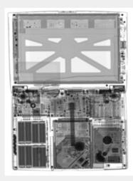
X-ray irradiation time is very short so electronic component damage is held to an absolute minimum during inspection. The high dynamic range of the camera detects a wide range of brightness distributions in one shot. Images of various objects ranging from low-density members such as resin and thin aluminum to high-density members such as batteries, HDD and CD drive structures can be acquired at the same time.
