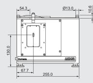
Optics for transient absorption measurement C13406-11 (Approx. 18 kg)
