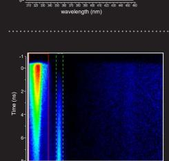
310 320 330 340 350 360 370 380 390 400 410 420 430 440 450 44 Wavelength (nm) Time-resolved transient absorption spectral streak image in simultaneous observation of the singlet-singlet absorption and the triplet-triplet formation of Anthracene solution
