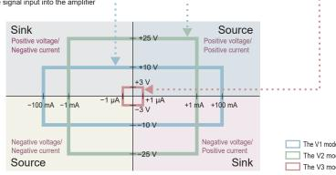
The V1 mode/The I1 mode measurement range The V2 mode measurement range The V3 mode measurement range
