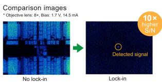
High S/N is achieved by acquiring signals at a specific frequency and eliminating signals at other frequencies as noise.
