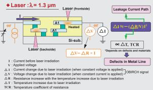
The OBIRCH amp can work for devices, which need to apply four quadrants of voltage/current. V1 mode, I1 mode, V2 mode, and V3 mode are selectable via software.
