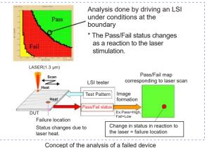
by utilizing the "drive voltage – operating frequency" characteristics
