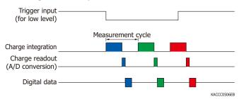
In any of the modes 1 to 6, if the trigger input cycle is shorter than the measurement cycle of the spectrometer, the input trigger is ignored.
