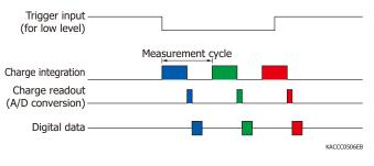
In any of the modes 1 to 6, if the trigger input cycle is shorter than the measurement cycle of the spectrometer, the input trigger is ignored.
