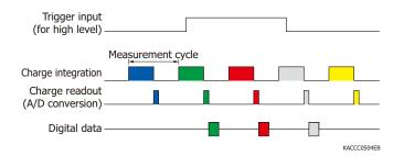
(4) Synchronous data measurement at external trigger input
