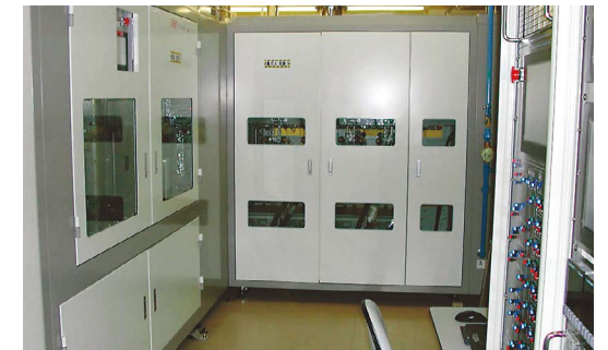
Thin-film crystal growth with MOCVD equipment
