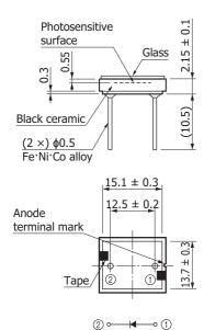
Chip position accuracy with respect to the package center  $-0.3 \le X$ ,  $Y \le +0.3$
