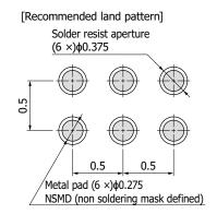
Tolerance unless otherwise noted:  $\pm 0.05$  Solder bump material: Sn (96.5%), Ag (3%), Cu (0.5%)
