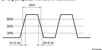
Output optical waveform definition
