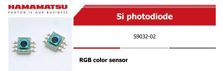
The S9032-02 is a color sensor molded into a plastic package having a 3-channel (RGB) photodiode sensitive to the blue ( $\lambda p$ =460 nm), green ( $\lambda p$ =540 nm) and red ( $\lambda p$ =620 nm) regions of the spectrum. The S9032-02 has a 3-segment (RGB) circular photosensitive area of  $\phi 2$  mm.
