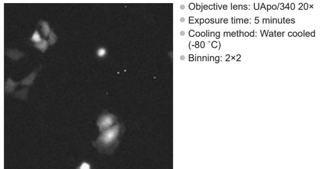
An often overlooked benefit of EM-CCD technology is the ability to utilize the camera as a standard CCD. In non-EM mode, there is no effect of excess noise, and the large full well capacity and high dynamic range are ideal for bright light applications that have large intrascene dynamic range. The ImagEM X2 series provides a low read noise non-EM mode that can be an ideal choice for such applications.
