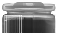
Possible to inspect the mismatch of rolling and measure the length of electrode with no distortion.
