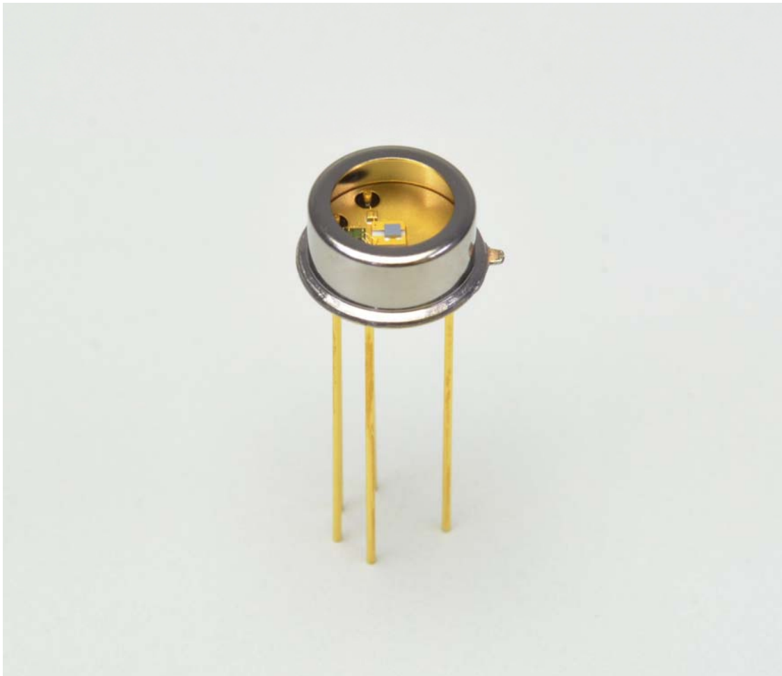
InAsSb photovoltaic detector with preamp P16702-011MN
