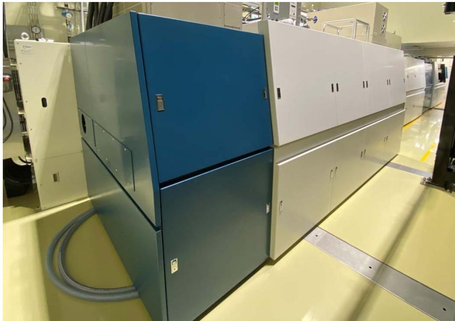
Fig. 3 External view of 250-joule industrial pulsed laser
