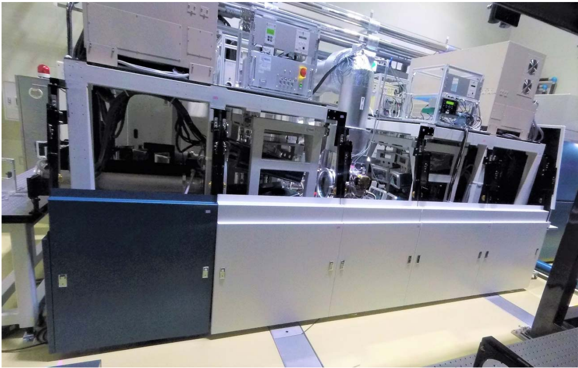
External view of the laser system producing laser pulses of 100 J at 10 Hz
