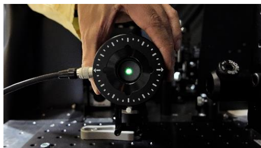
Observation of THz wave beams using THz I.I.
