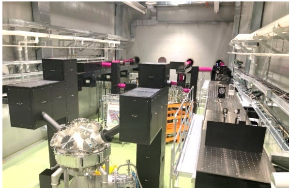
Hamamatsu Photonics laser fusion experiment facility and an experiment chamber owned by EX-Fusion
