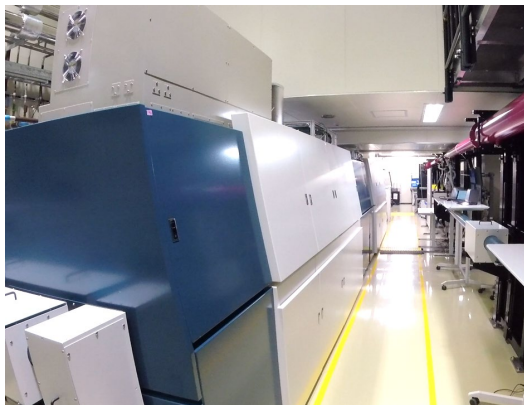
Hamamatsu Photonics LD-pumped laser generating the world's highest power (HALIANS) [4]
