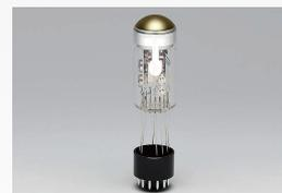
▲ Photomultiplier tube used in the Cherenkov Telescope Array (CTA)
