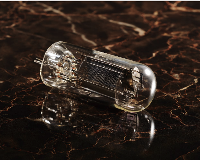
▲ Our first side-on photomultiplier tube type R105 in 1959
