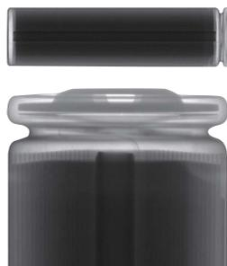
Internal shape inspection of Li-ion batteries
