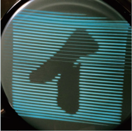
1926 Prof. Takayanagi succeeded in receiving images on the world's first electronic cathode-ray tube. 「イ」 is derived from the “Iroha” order as the first character of the traditional Japanese syllabary. (The photograph is of the reproduction device.)
