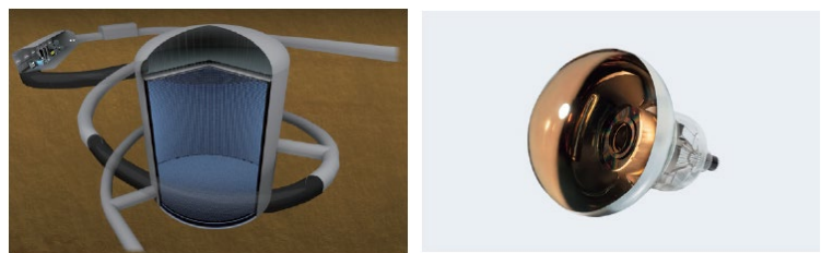
▲ Conceptual diagram of “Hyper-Kamiokande,” the next-generation of neutrino measurement experiments (left. Photo courtesy of the Kamioka Observatory, Institute for Cosmic Ray Research, The University of Tokyo). A PMT (right) is attached to the tank wall in the center.
