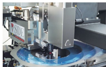
▲ Stealth Dicing Engine (left) and a laser beam is used to create cracks in the wafer to cut it (right).
