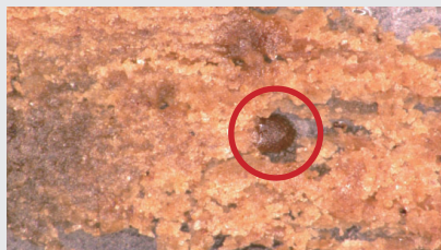
▲ Laser irradiation on chocolate slice Laser beam setting: \Phi 80 \mu\text{m} Irradiation marks: \Phi 170 \mu\text{m}
