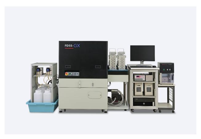
Another key benefit is its high sensitivity achieved through the integration of Hamamatsu's renowned qCMOS sensor, which is incorporated into the world's first photon-resolving camera. It enables high-quantitative performance for low-light imaging, useful for fluorescence and luminescence measurements. Additionally, it provides a larger resolution and field of view, pushing the limits in terms of measurement accuracy.
