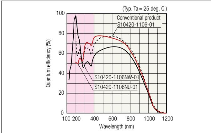
Variation in the spectral sensitivity due to UV light irradiation
