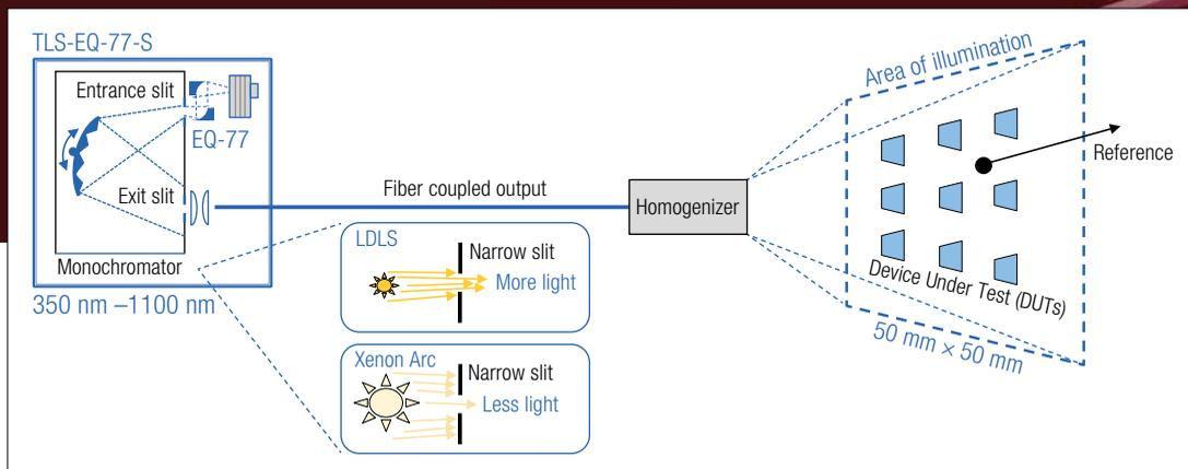
Figure 1: A tunable broadband source is used to calibrate ambient light sensors.
