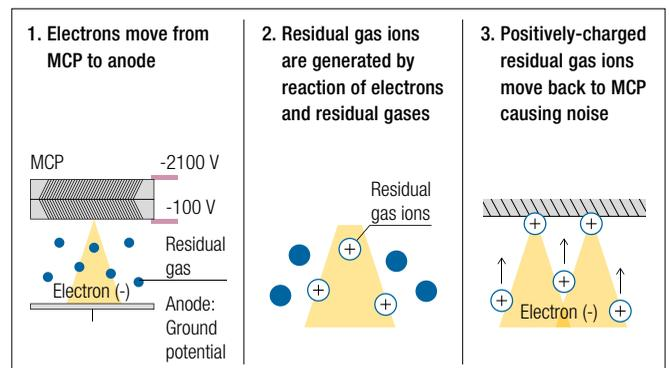
“ion feedback” (in figure 3). When ion feedback occurs, the residual gas ions collide with the channel walls of the MCP and cause the emission of electrons. These electrons are then multiplied in the MCP channel walls generating noise signals. If these noise signals increase, they will disturb and degrade the high sensitivity and accuracy of the measurements required for mass spectrometry.
