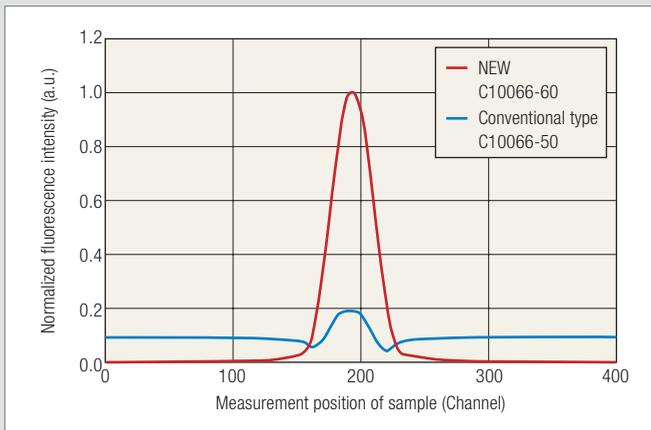
**Matsumura:** In addition to improving sensitivity, we upgraded other components. For example, we redesigned the lens of the optical system to enhance the beam focus and also modified complex algorithms for the digital section. I suppose the total result from all these small modifications contributed to enhancing the overall sensitivity.
