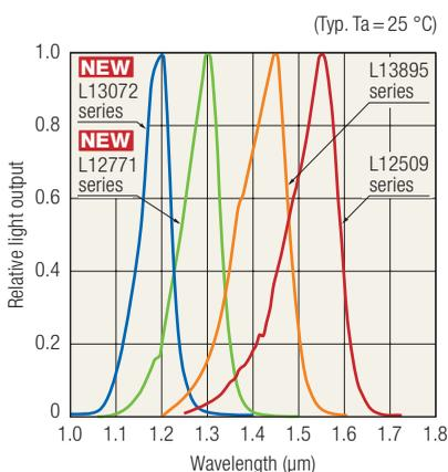
We have a lineup of near infrared LEDs that support various wavelength bands (1.2  $\mu\text{m}$ /1.3  $\mu\text{m}$ /1.45  $\mu\text{m}$ /1.55  $\mu\text{m}$ ). In addition to the surface mount type, we also offer a highly reliable metal package and a narrow directivity bullet type.
