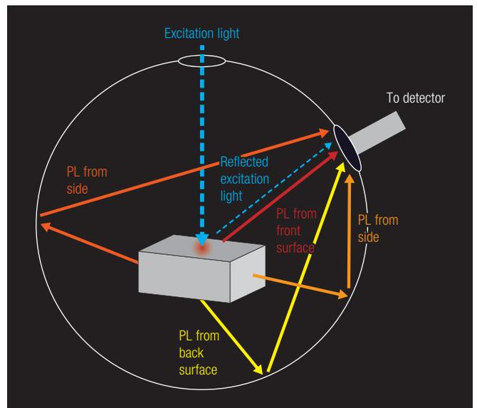
Averages and detects PL emitted not only from the front surface irradiated with excitation light but also from the back surface and sides after being absorbed or transmitted inside the crystal.
