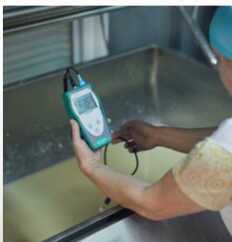
MEASUREMENT OF MOISTURE CONTENT TO MONITOR CHEESE MATURITY
