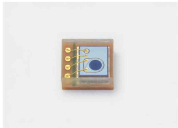
Hamamatsu's Si Avalanche Photodiode series S15415.
