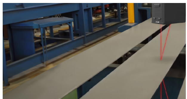
Image 1: Non-contact measurement of material thickness.
