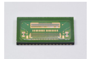
Hamamatsu photosensor S14137-01CR including a 16-element APD array.
