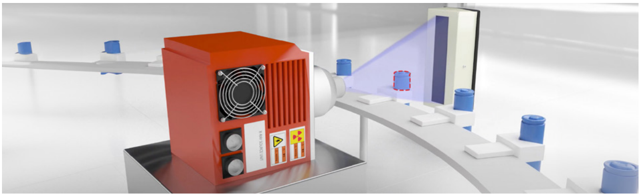
Figure 1: Conceptual representation of in-line cylindrical battery inspection setup using a sealed-type Hamamatsu microfocus X-ray (MFX) source and a time delayed integration (TDI) camera.
