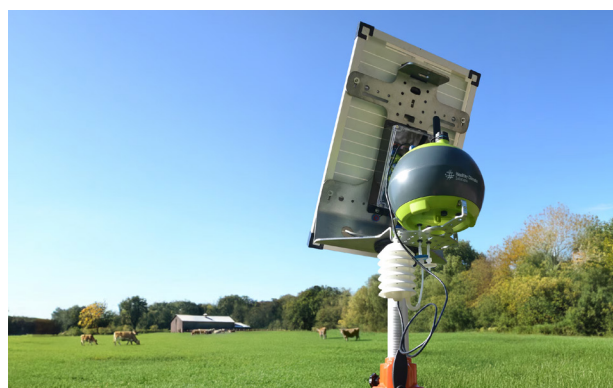
Continuous CH 4 emission monitoring around barns (Axetris)
