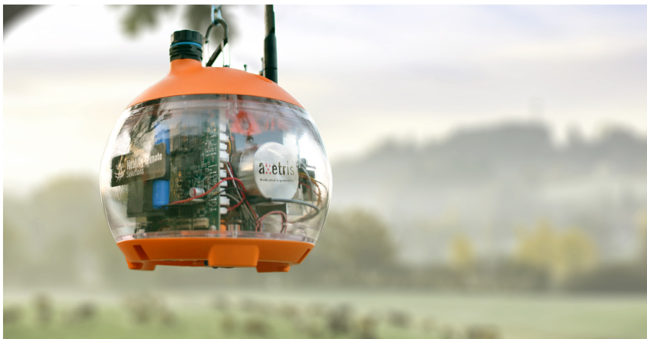
Axetris' integrated LGD Compact CH 4 for outdoor CH 4 monitoring
