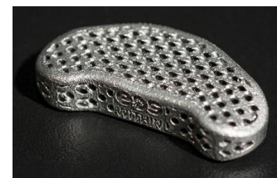
3D printing by laser powder bed fusion
