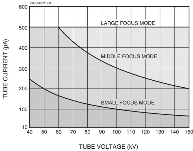
\* The X-ray tube voltage guaranteed range is 40 kV to 150 kV.
