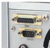
Upper: D-sub connector Under: RS-232C
