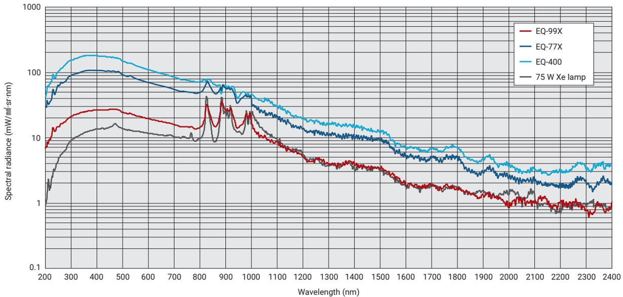
\* We have confirmed wavelength radiation from 170 nm to 2500 nm, but we have not acquired the wavelength band Less than 200 nm and after 2400 nm for spectral radiance data.
