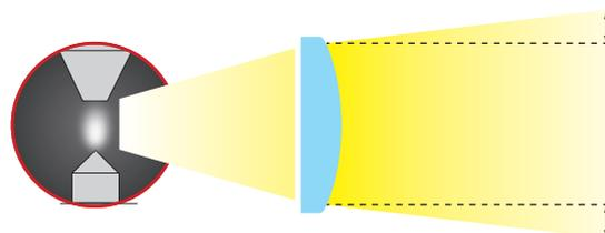
When collimating light from traditional light sources, the beam divergence or widening angle usually becomes a problem. LDLS allows forming ideal collimated light with a smaller divergence angle than xenon lamps. The small emitting point is also advantageous for efficiently focusing the light onto a very small area.
