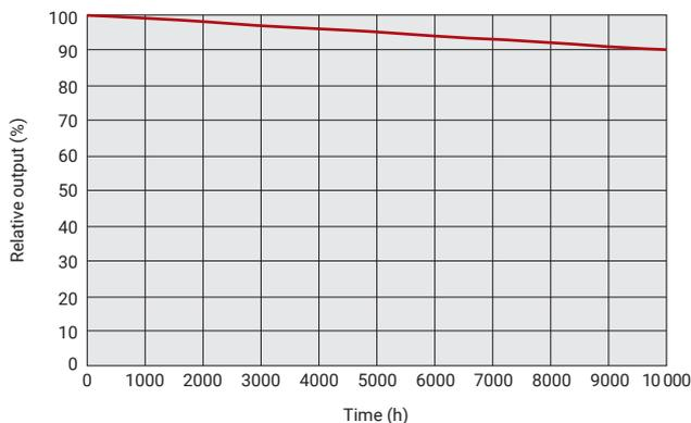
\* This is the typical lifetime of EQ-99X-QZ-S measured light output at 500 nm.
