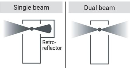
A retroreflector is attached to the lamphead (standard feature) on the EQ-77X-QZ-S and EQ-400-RH-QZ-S LDLS for single-beam output mode. Light reflecting from the retroreflector combines with the light directly emitted from the bulb to enhance the output in one direction. Removing the retroreflector allows light emission in two directions for dual-beam output mode.
